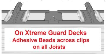
Note:- Insertion of boards into the clips must be done within 5 mins of applying adhesive to ensure correct adhesive properties.
