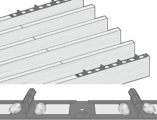
Adhesive applied as "Dobs". Natural Grain Collection Boards Inner Joists only
