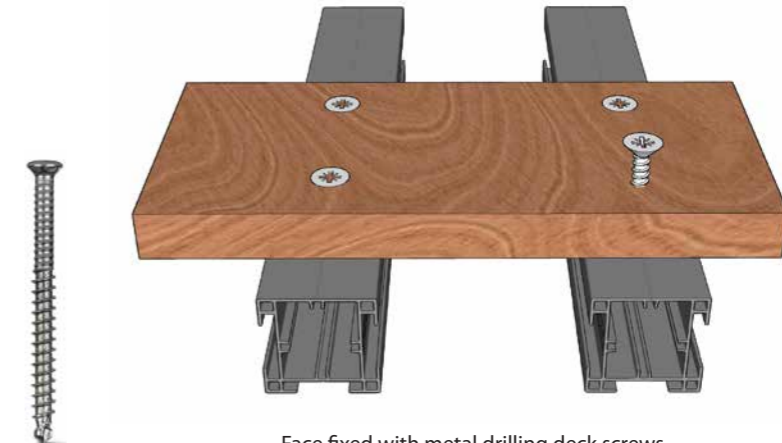
Face fixed with metal drilling deck screws
